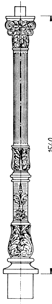
THK-610-K Candelabra top part with Spigot \varnothing 60 mm or flanged connections Weight: approx 51 kg
